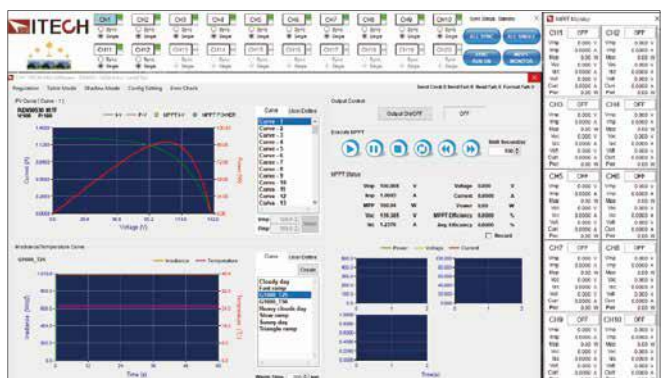
Multi-channel MPPT test
